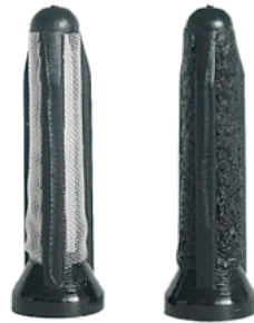
Prefilter of the E1F: new on the left, blocked on the right
