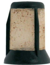
Prefilter of the E3T – blocked by rust
